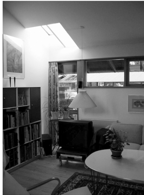
Space 2 – horizontal windowpanes in both outer walls, sloped ceiling, no level differences, reverberation time 0.6 seconds
