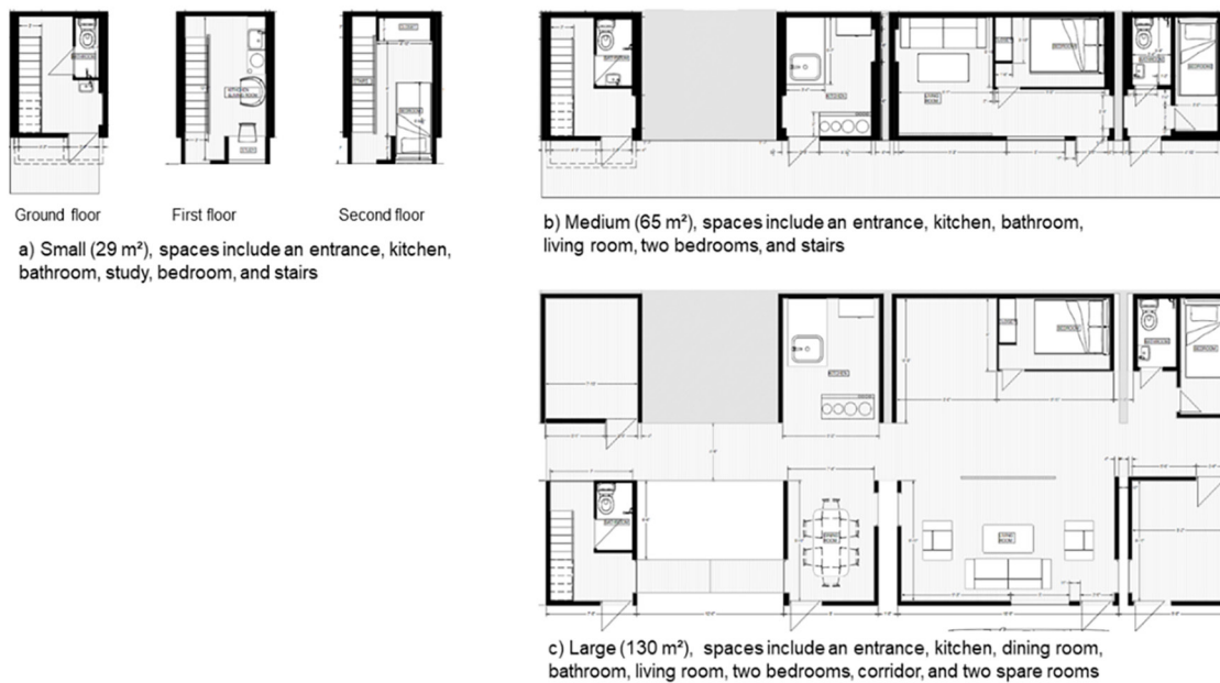
Figure 6 Floor plans of the small (a), medium (b) and large (c) micro units proposed
