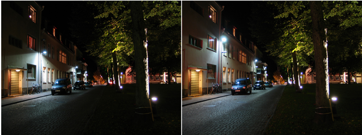
Figure 3 The temporal street luminaires had varying heights (4.5 m on the left and 6 m on the right).
