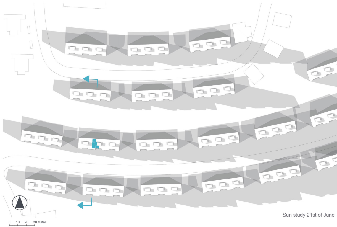
Figure 5 a A case study from the 1960s; sun study at 9.00, 12.00 and 15.00 on the 21 st of June.
