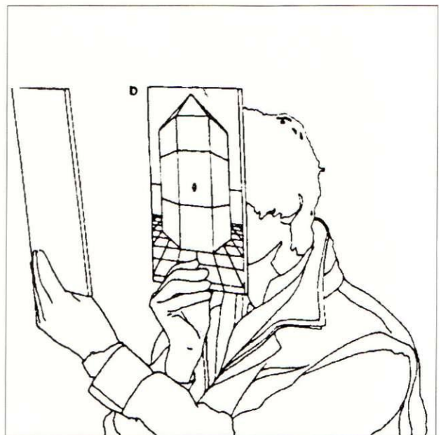
Brunelleschi's two-panel system for viewing a perspective drawing. Courtesy Kevin Forseth.
