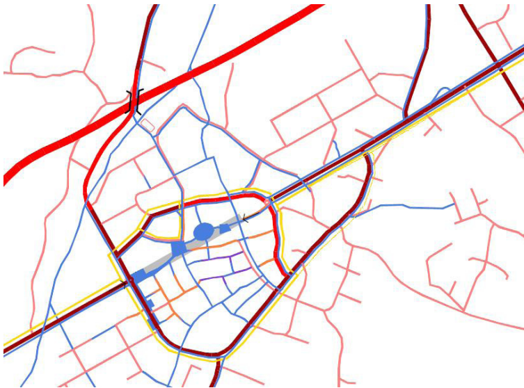
Drawing 6. Road network, illustration of the conflict between the historical road line and the By och mur -solution. The straight line of the main road has been replaced with a series of open public spaces, whereas the other road is preserved as a curve around the centre.
