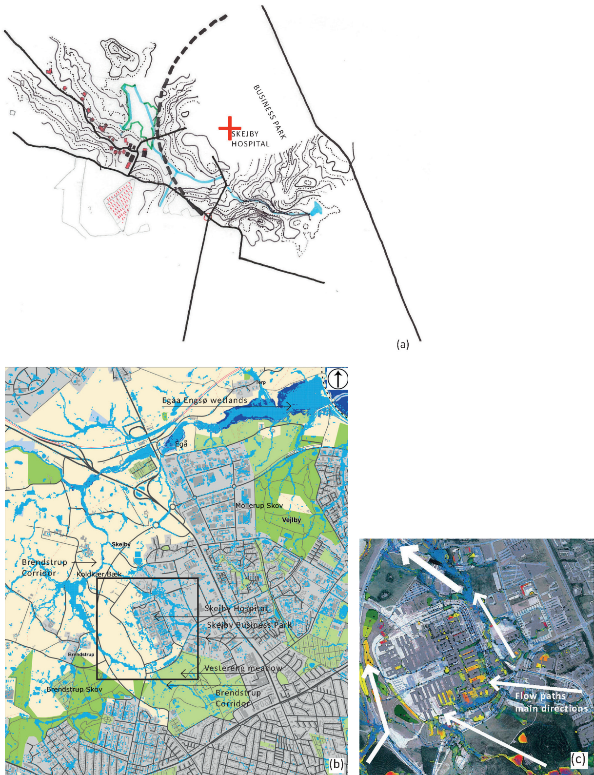
Figure 3.2.2 Flood risk projection of the Region's largest hospital and relations to the larger landscape characteristic of the deep structure Brendstrup Corridor, starting south of the Business park, passing the hospital and Egå Engsø on its way to the sea. (a) tracing of contour lines and surface water from the late 19th Century map indicating the overall direction of the terrain and surface water. (b) flood risk projection on contemporary map (c) flood risk projection Skejby Hospital with a diagrammatic marking of flow-paths' direction on aerial photo, 2014. Source: (a) SDFE (b) SDFE, Aarhus Kommune, Klimatilpasningsplan 2014, (c) Aarhus Kommune.
