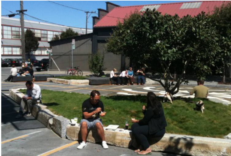
Figure 5 Showplace Triangle Plaza during the Pavement to Parks Trial period. Reused kerbstones and granite blocks create islands for sitting between two restaurants.
