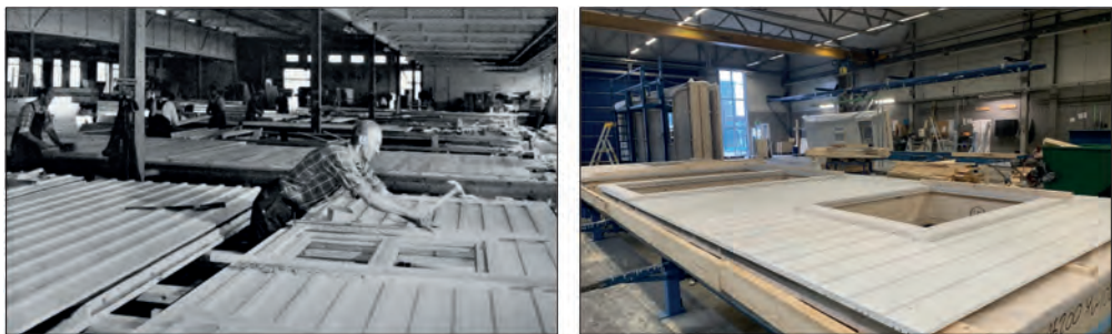
Figure 1. Swedish prefab manufacturing process in the past and present. The image on the left was taken in 1951 inside Åmål's Sågverks Aktiebolag, whereas the one on the right was taken in 2019 inside the A-hus Factory.
